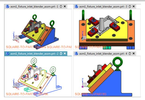
The concept of the main and secondary windows is also no longer valid. NX treats all open windows of a construction the same. A part is not closed until you close the last window that displays that part. In earlier versions of NX, all windows created with the New Window command are called secondary windows. When the primary window is closed, NX automatically closes the secondary windows associated with the primary window.
